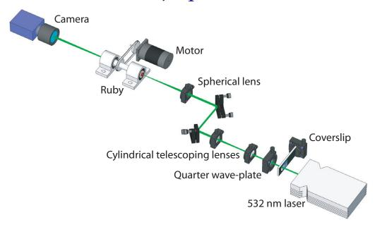
**Figure 2.** Experimental procedure. A beam of 3 W, 532 nm light is bisected by a coverslip. The entire beam then passes through a quarter waveplate, two cylindrical telescoping lenses and is focused on a ruby window. The ruby is spun to  $\approx \pm 20$  rotations per second (rps), and the light leaving the ruby is imaged onto a camera.
